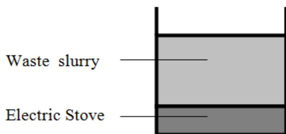
Fig. 1. Hydrolysis Equipment
