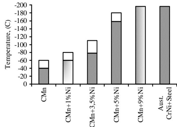
Fig. 1. Operating temperatures for different steel grades
