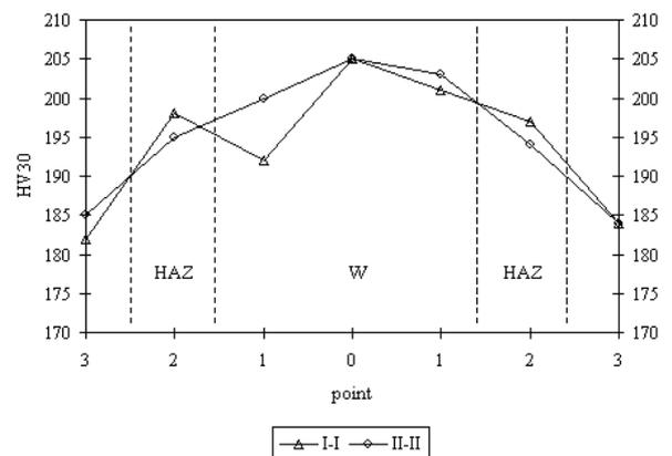
Fig. 10. HV30 hardness variation of welded seam
