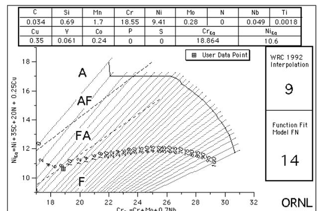
Fig. 2. WRC diagram for determining the structure and δ ferrite content of 321 steel
