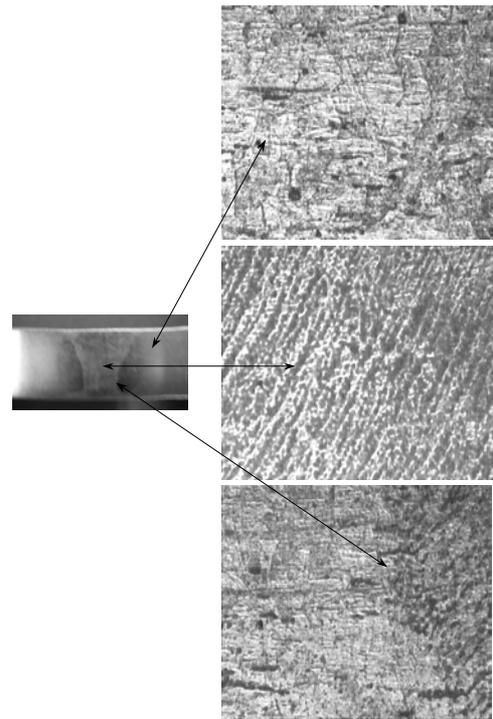
Fig. 9. Macro and microstructure of sample. Attack: aqua regia. 200:1
