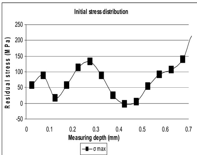
Fig. 5. Residual stresses distribution before milling
