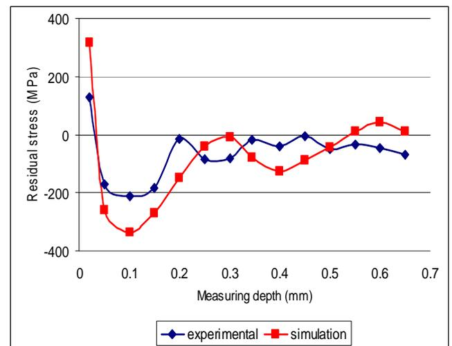
Fig. 13. Residual stress distribution generated by a double cutting regime (V2 + V3)
