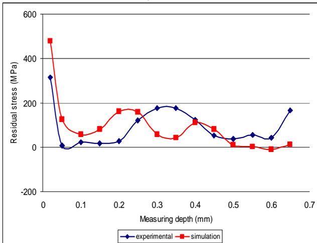
Fig. 10. Residual stress distribution generated by V 250 m/min and 0.25 mm depth
