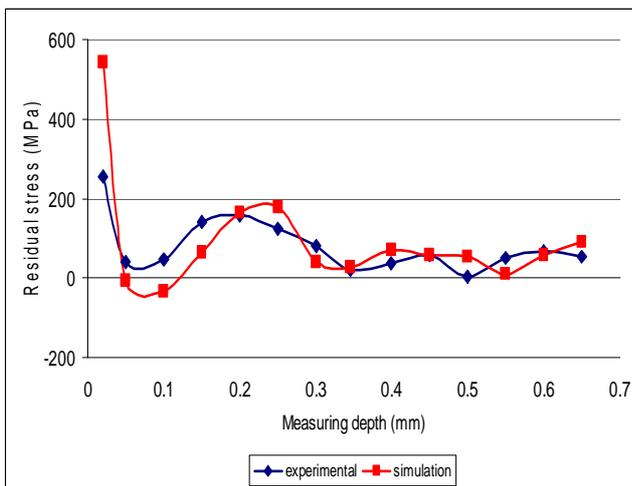
Fig. 11. Residual stress distribution generated by V 1036 m/min and 0.15 mm depth
