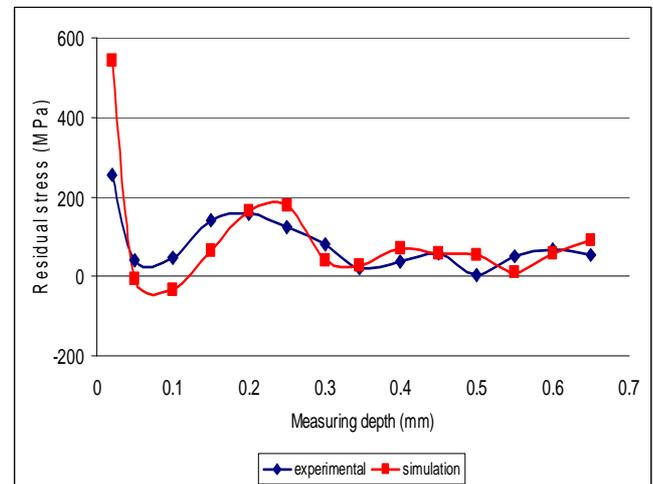
Fig. 12. Residual stress distribution generated by a triple cutting regime (V1 + V2 + V3)
