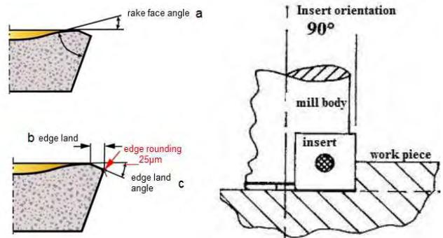
Fig. 3. Geometry of milling insert and orientation of cut
