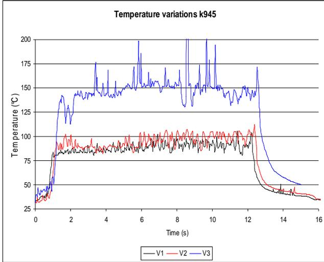
Fig. 7. Temperature variations when milling with different cutting speeds
