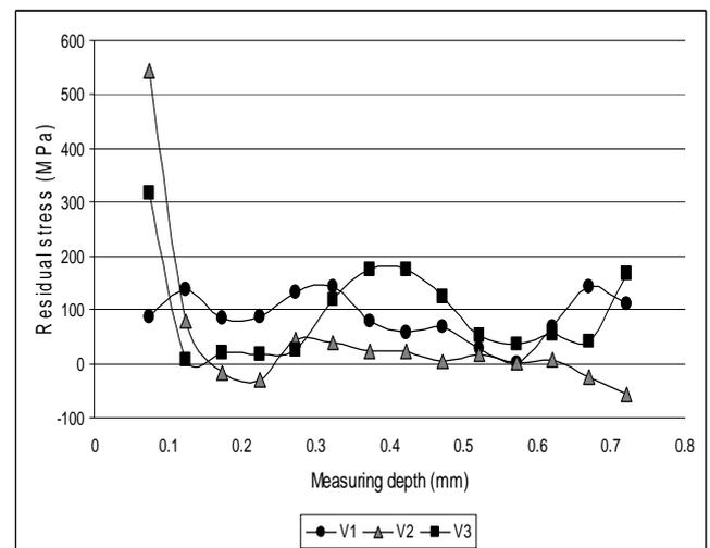
Fig. 6. Residual stresses distribution generated by milling operation on separate materials
