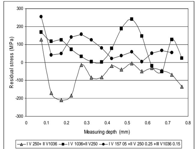
Fig. 8. Residual stress distribution generated by successive milling operations
