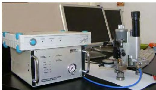
Fig. 1. Hole-drilling residual stress measuring equipment
