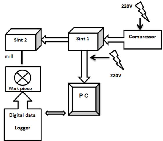
Fig. 2. Schema of the hole-drilling residual stress measuring method [11]
