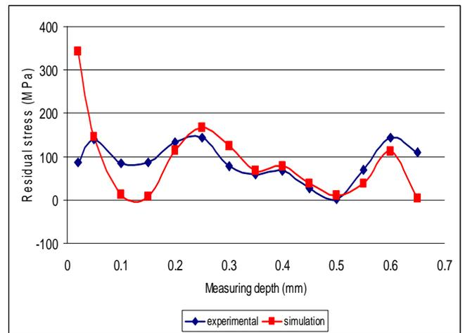
Fig. 9. Residual stress distribution generated by V 157 m/min and 0.5mm depth
