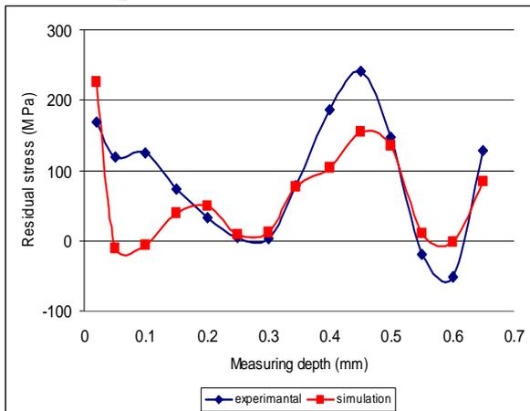
Fig. 14 Residual stress distribution generated by a double cutting regime (V3+V2)
