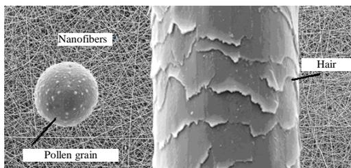
Fig.1. SEM image of a hair vs. pollen grain vs. nanofibers
