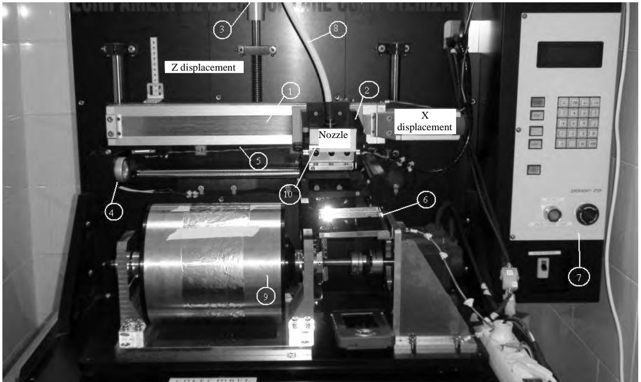
Fig.3. Computerized electrospinning equipment, [10]
