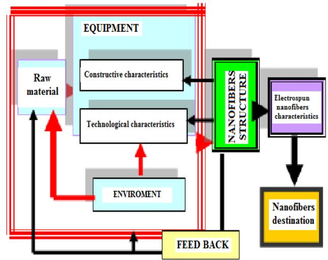
Fig. 2. Factors which influence the characteristics of the electrospun nanofibers, [8]
