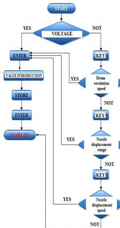
Fig. 11. Diagram for setting the technological parameters on the ELECTROSPIN equipment, [10]
