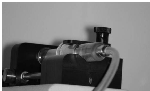
Fig. 5. Position of the syringe on the delivery pump, [10]
