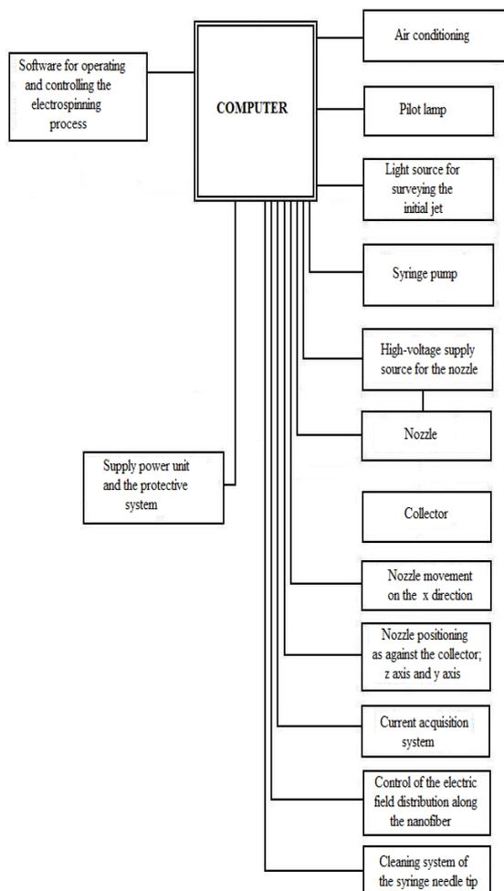
Fig.9. Diagram of the computerized components, [9]
