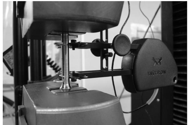
Fig. 8. Tensile test set-up
