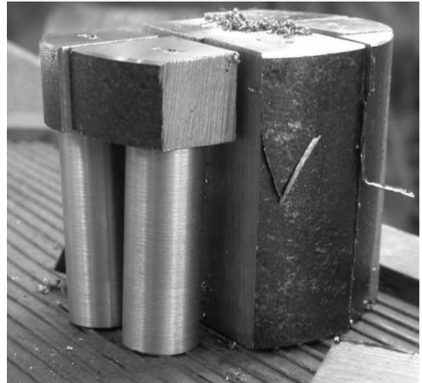
Fig. 7. Division of the steel bar
