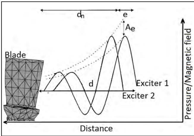
Fig. 3. Exemplification of speakers position deviation that can produce amplitude and phase errors in the excitation
