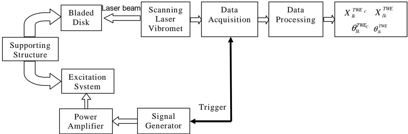
Fig. 1. Measurement experimental setup
