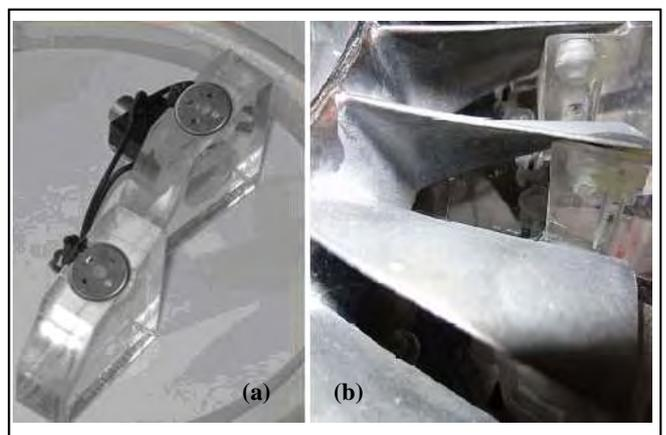
Fig. 2. (a) Speakers mounted on plastic fixtures; (b) Speakers positioned to lie parallel to the blade faces
