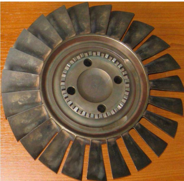
Fig. 5. The 23-industrial bladed disk used in the experimental testing
