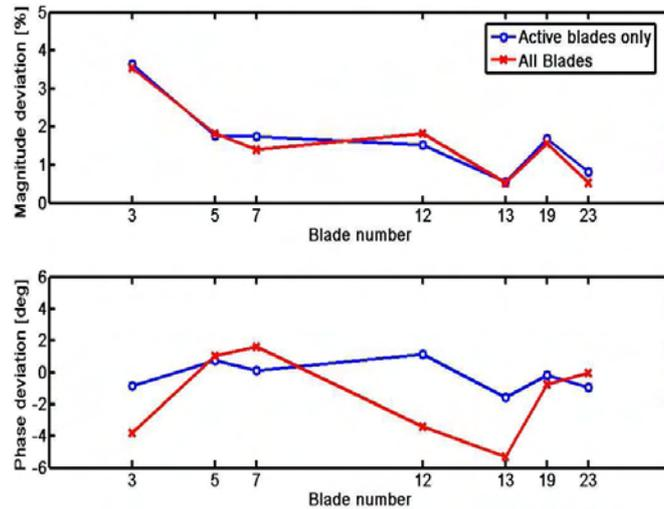
Fig. 6. Experimental results from two different cases of the novell TWE procedure for an engine-order-excitation 1 at the resonant frequency of 4100Hz of the first torsion family mode, for nine blades of a 23 industrial bladed disk
