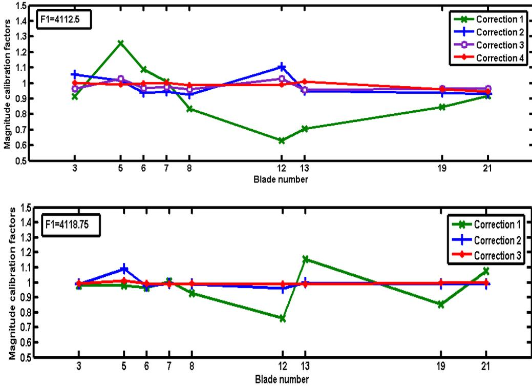
Fig. 4. Experimental results from four iterations of the calibration procedure for an engine-order-excitation 0, at three resonant frequencies of the first torsion family mode, for nine blades of a 23 industrial bladed disk
