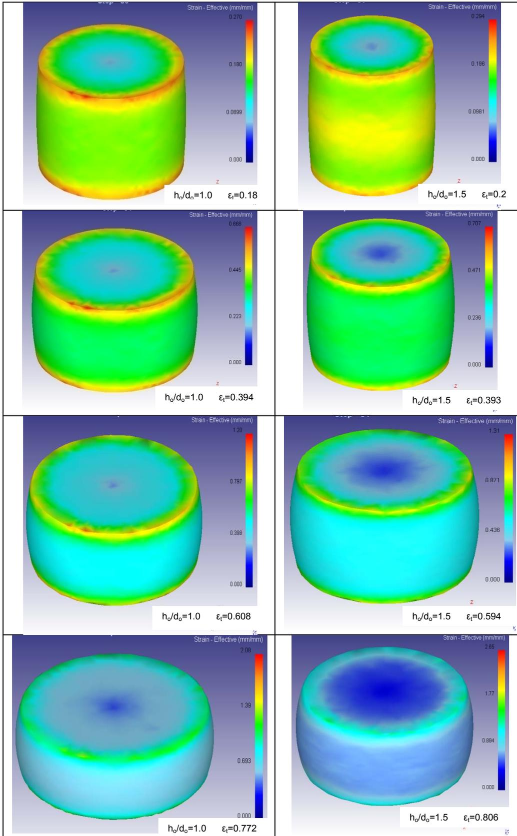
Fig. 3. Strain distribution of the billet with different deformation degrees
