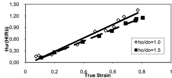
Fig. 10. The variation of  $H_{ur}$  with the aspect ratio
