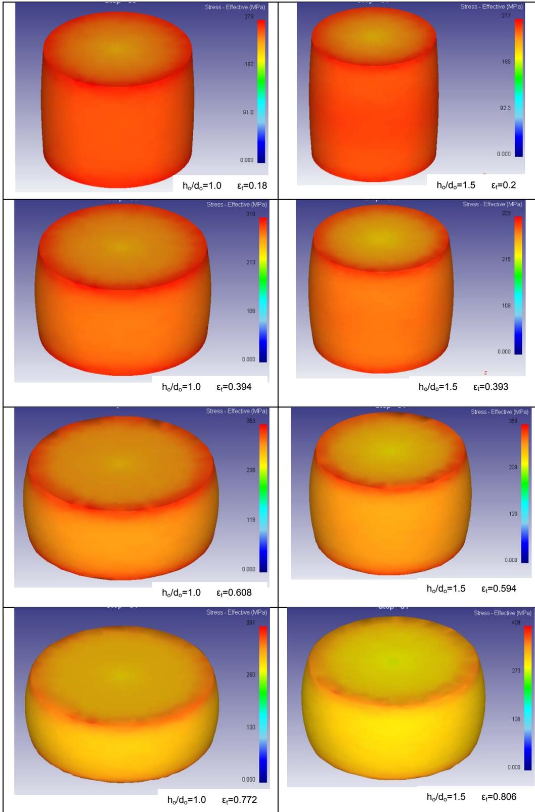
Fig. 4. Effective Stress distribution of the billet with different deformation degrees
