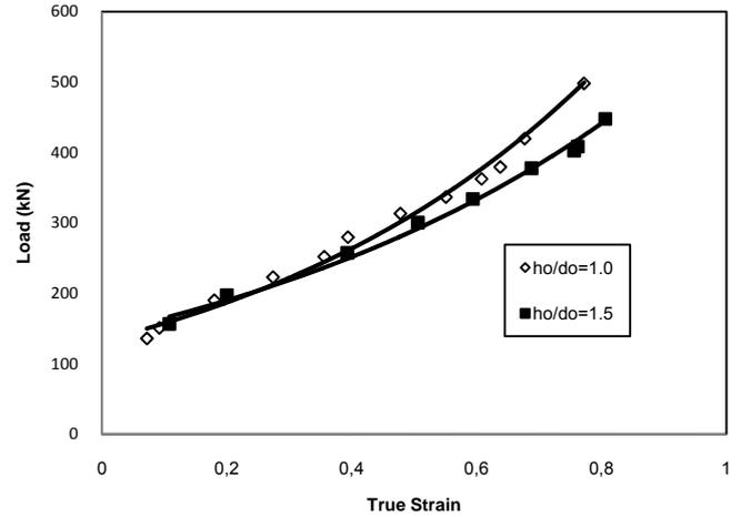
Fig. 2. Variation of load versus true strain
