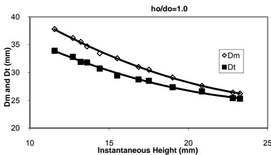
Fig. 8. Change of maximum and top diameter versus height of cylinder during deformation for  $h_0/d_0=1.0$
