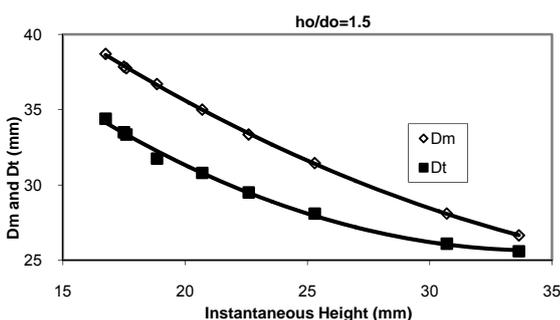
Fig. 9. Change of maximum and top diameter versus height of cylinder during deformation for  $h_0/d_0=1.5$
