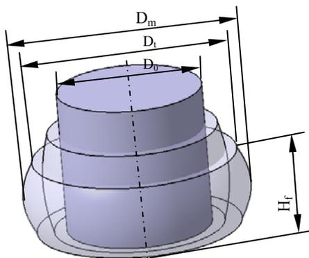
Fig.1 Barreling profiles at different stages and related dimensions.
