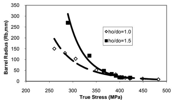
Fig.7. The variation of the barrel radius with the true stress
