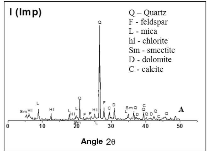
Fig. 2. X- ray of raw material
