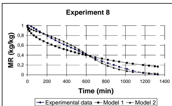
Fig. 12 – Drying results for experiment 8
