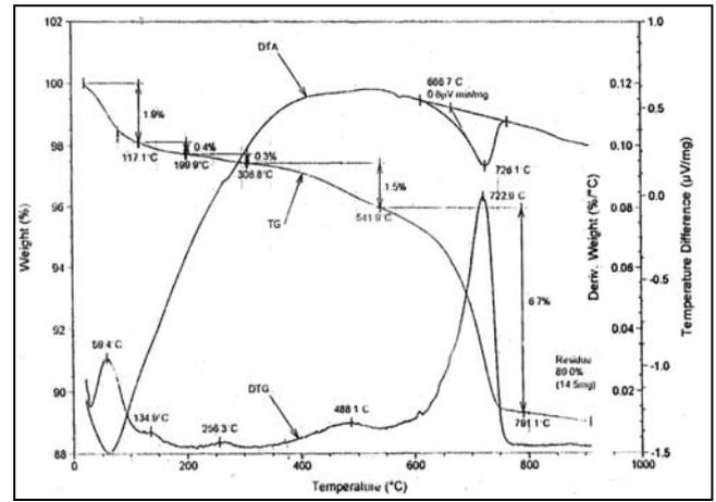
Fig. 3 - DTA and TGA of raw material
