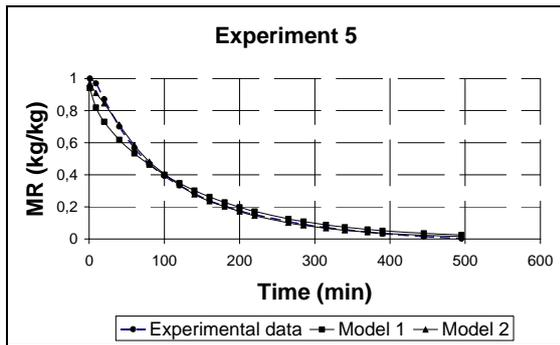
Fig. 9 – Drying results for experiment 5
