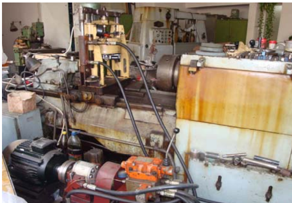
Fig.3. The entire rotorolling equipment
