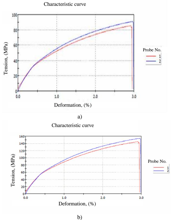
Fig.10. The characteristics curve: a-base alloy; b- composite material obtained
