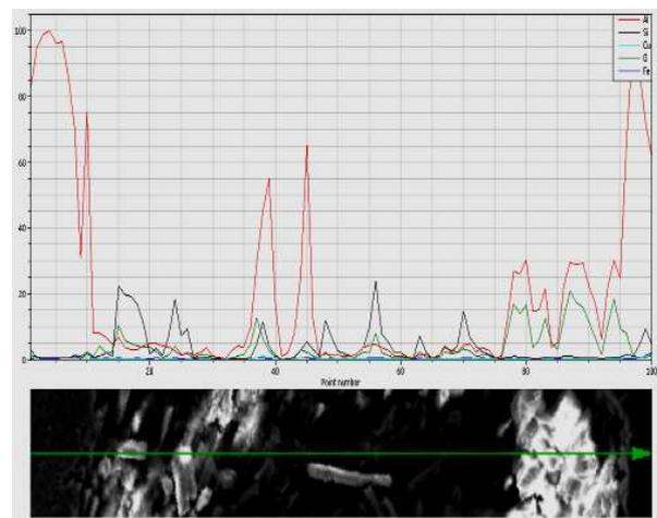
Fig. 12. Variation of content of elements in the matrix and glass fibers
