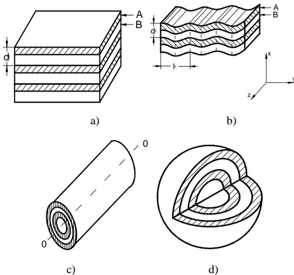
Fig. 2. Types of laminated composite with regular structure:
