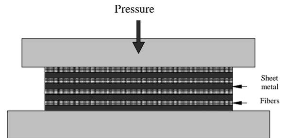
Fig. 3. Engineering merge by diffusion of continuous fiber composites
