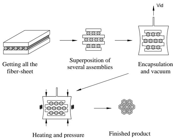
Fig. 5. The combining diffusion scheme to obtain metal matrix composites
