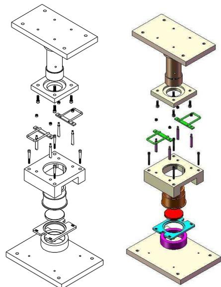
Fig. 7. The general scheme of the mold assembly
