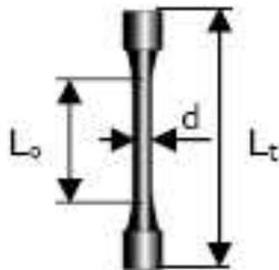
Fig. 9. Standard test-piece for tensile testing
