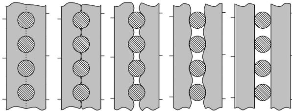
Fig. 4. The diffusion process scheme of consolidation of system fiber - film
