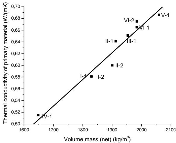
Fig. 3. Primary material thermal conductivity as a function of net volume mass
