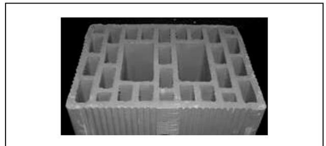
Fig. 2. Hollow block without thermal bridges (sample I-2)
