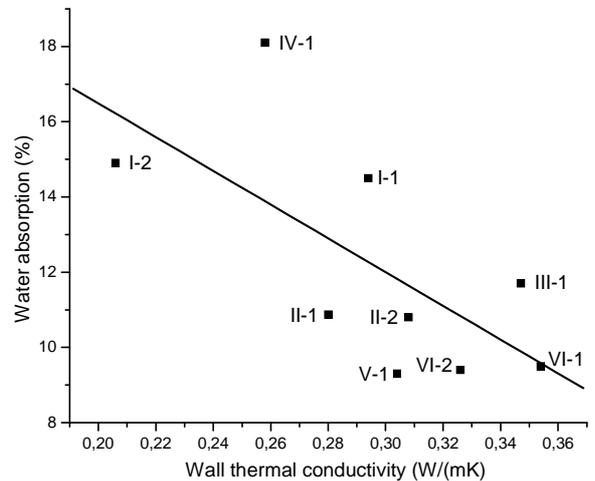
Fig. 6. Wall thermal conductivity as a function of water absorption
