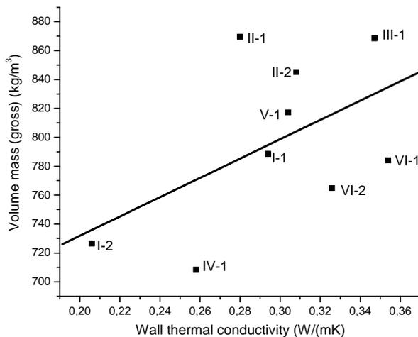
Fig. 4. Wall thermal conductivity as a function of gross volume mass
