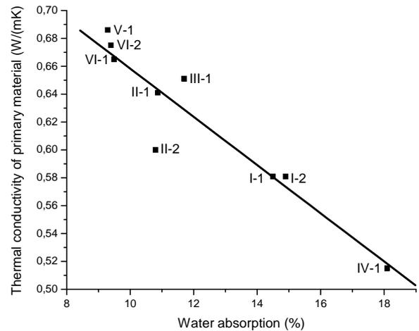
Fig. 5. Primary material thermal conductivity as a function of water absorption
