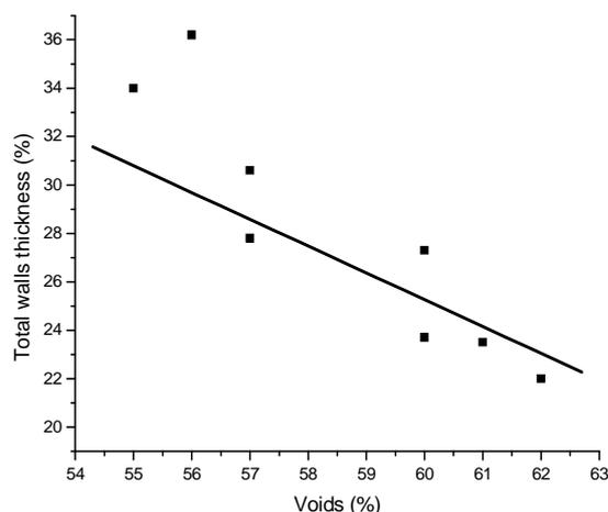
Fig. 8. Relation between total wall thickness and voids fraction
