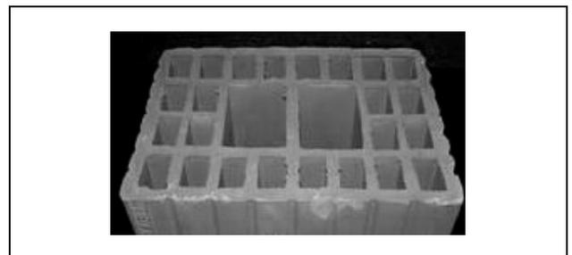
Fig. 1. Hollow block with thermal bridges (sample VI-2)
