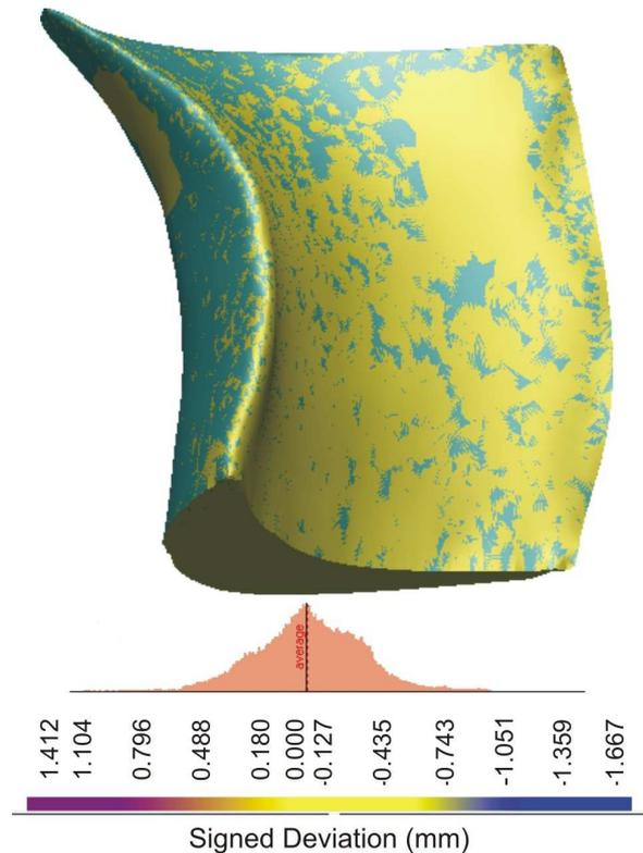
Fig. 6. Two point clouds deviation after the automatic registration process of the wing
