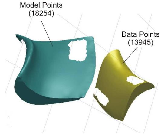
Fig. 3. Initial position of point clouds with the same boundaries and different holes
