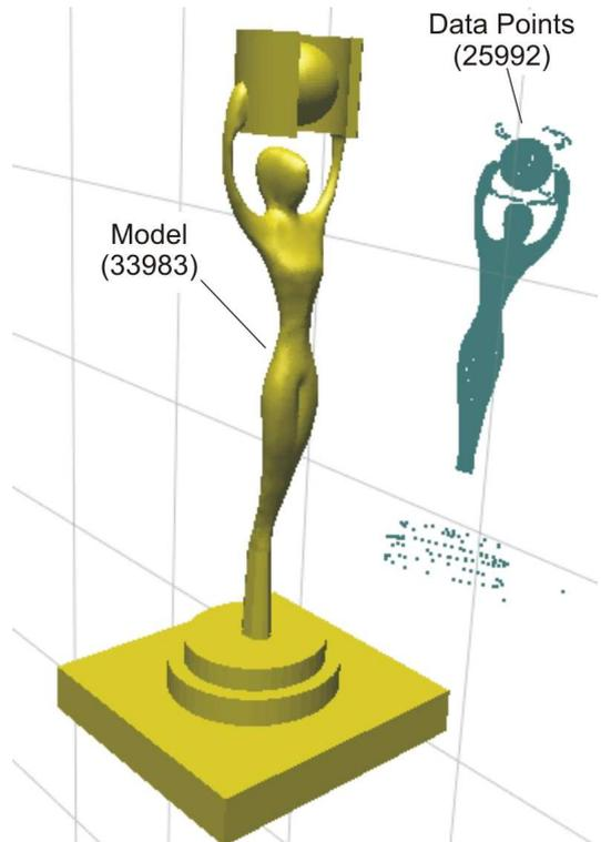
Fig. 4. Initial position of a CAD model and a point cloud
