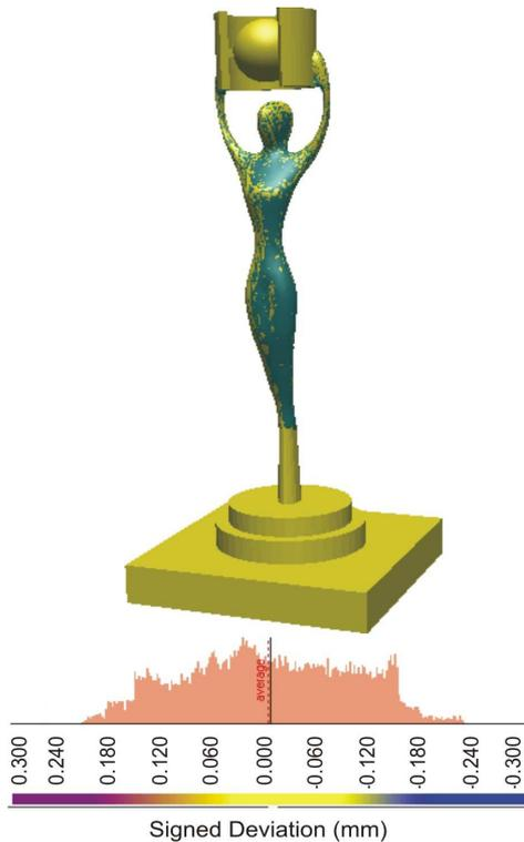
Fig. 7. Two point clouds deviation after the automatic registration process of EUSY statue
