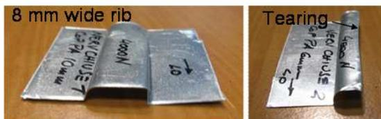
Fig. 19. Straight ribs formed by SBR shaped dies
