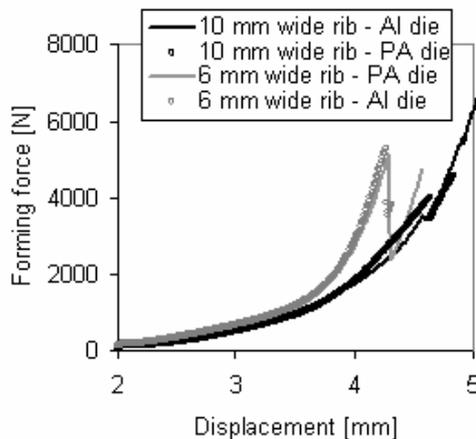
Fig. 18. Forming curves for straight ribs with shaped SBR upper dies and lower aluminium (Al) and PA dies
