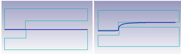
Fig. 23. Numerical analysis of straight rib forming: initial stage (left) and during forming (right)
