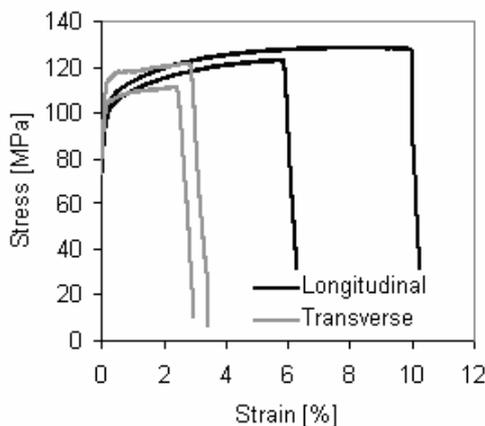
Fig. 2. Effect of the aluminium sheet direction on the tensile tests
