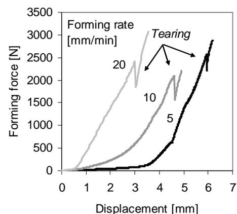
Fig. 11. Forming curves for conical cups with flat SR dies
