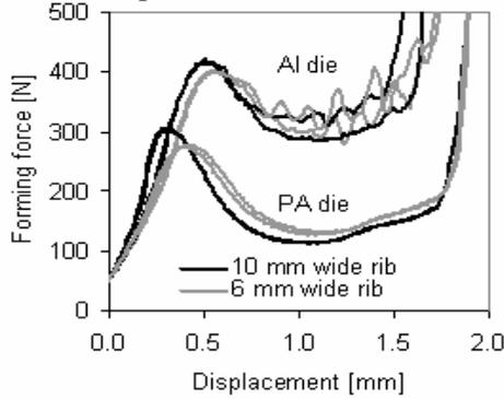
Fig. 20. Forming curves for straight ribs with shaped PA upper dies and different lower dies
