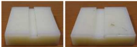
Fig. 7. PA lower dies for forming straight ribs: 6 mm (left) and 10 mm (right) width of the rib
