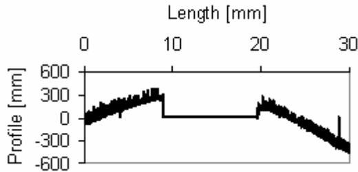
Fig. 22. Typical profile of a 10 mm wide rib formed with PA die
