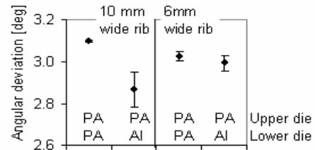
Fig. 26. Angular deviation of formed straight ribs by PA dies
