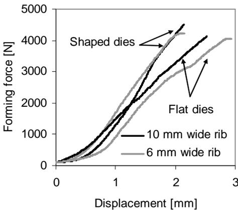
Fig. 14. Effect of die shape on forming curves for SR dies
