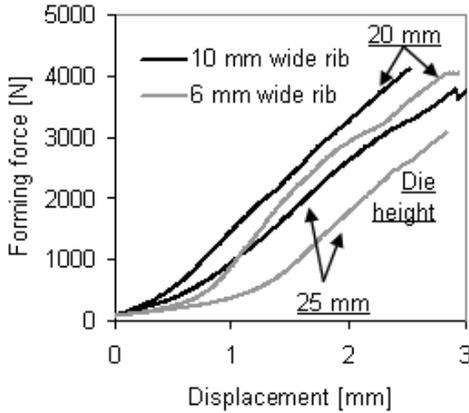
Fig. 13. Forming curves for straight ribs with flat SR dies
