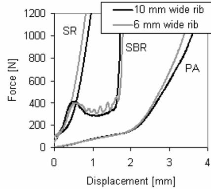
Fig. 25. A comparison between forming curves obtained with different die materials in the case of the 10 mm wide rib
