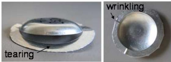
Fig. 12. Defects of formed cups by SR dies
