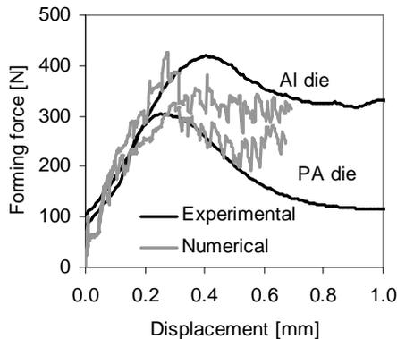
Fig. 24. Comparison between experimental data and numerical solutions for straight ribs
