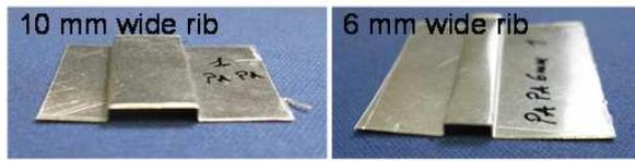
Fig. 21. Straight ribs formed by PA dies
