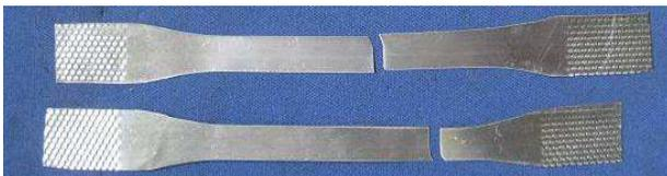
Fig. 1. Aspect of aluminium alloy specimens after tensile tests
