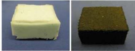
Fig. 6. An SR (left) and SBR (right) flat upper die for forming straight ribs
