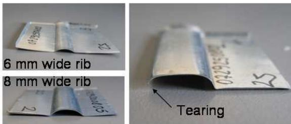
Fig. 15. Defects of formed straight ribs by SR dies
