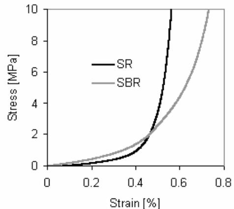
Fig. 4. Compression test of a SR and a SBR sample
