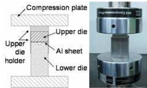
Fig. 9. Forming system for the straight rib
