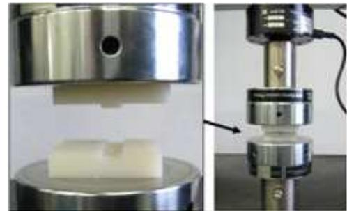
Fig. 10. Forming system with lower and upper PA dies
