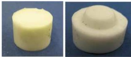
Fig. 5. SR dies: flat (left) and shaped (right) upper dies for forming conical cups
