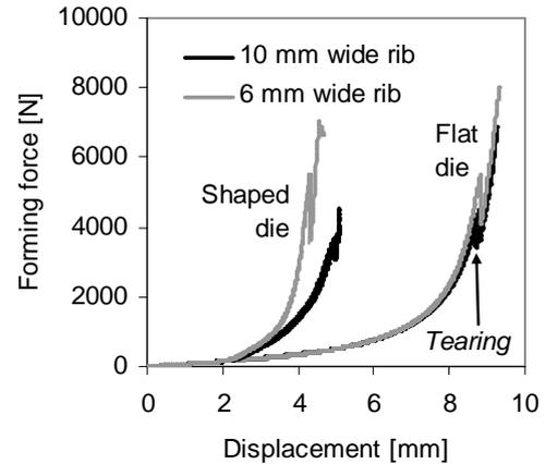
Fig. 17. Forming curves for straight ribs with flat and shaped SBR dies
