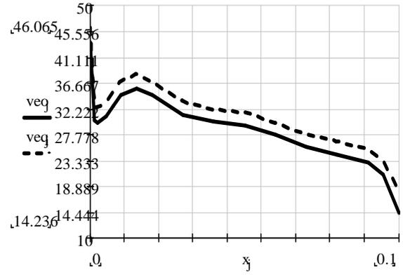
Fig. 4. Local speed distribution on upper side of wings
