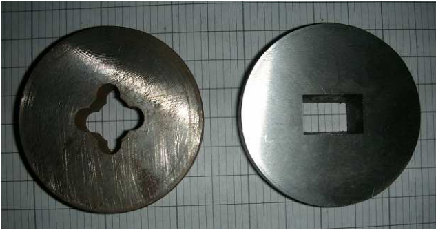
Fig. 1. A photographic view of clover and rectangular dies
