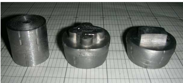
Fig. 2. Initial billet, clovered shaped work-piece and rectangular shaped work-piece
