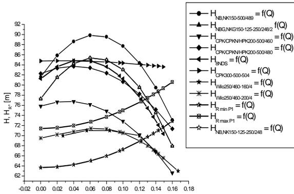
Fig. 1. Head variation depending on flow rate for pumps  $H = f(Q)$  and pipes network  $H_R = f(Q)$
