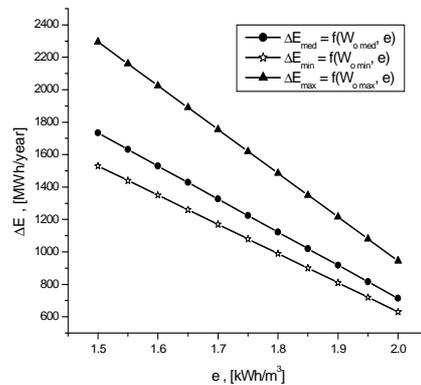
Fig.5. Electric power economy  $\Delta E$  depending on electric power specific consumption planned  $e$
