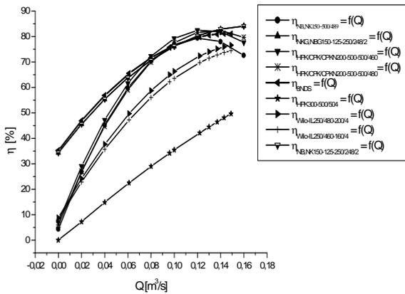
Figure 2. Outturn variation depending on flow rate  $\eta = f(Q)$
