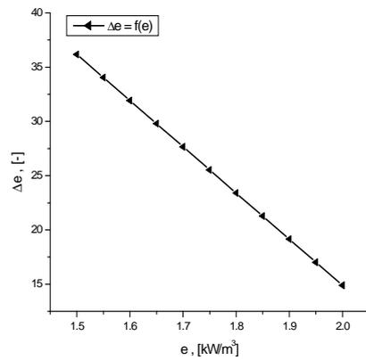
Fig.4. Energy consumption reduction  $\Delta e$  depending on electric power specific consumption planted  $e$
