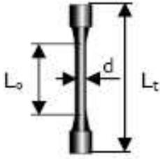
Fig. 2. Standard test-piece for tensile testing
