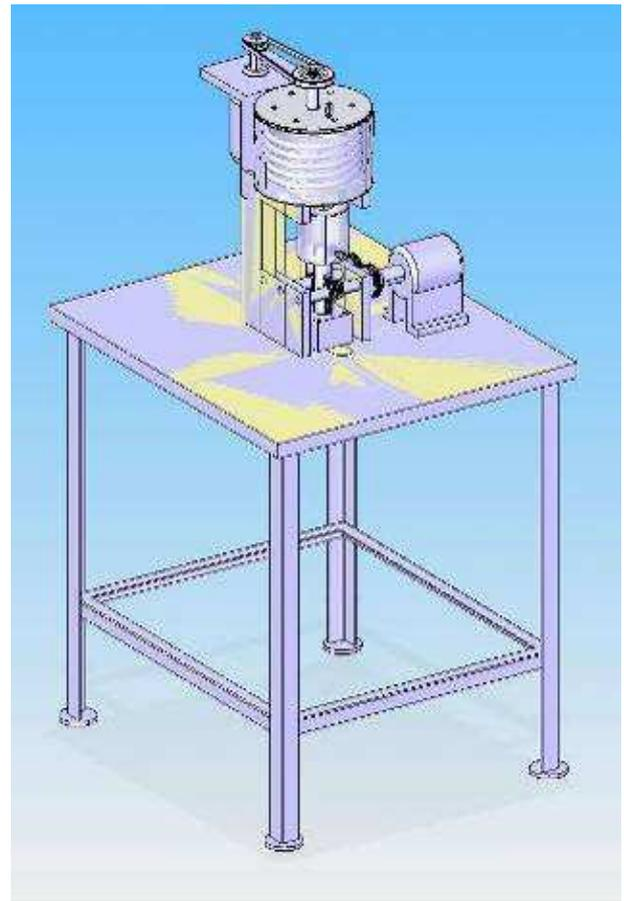
Fig. 1. The equipment for obtaining the composite material with mettalic matrix and particles reinforcement which is using the Vortex and semi continue casting
