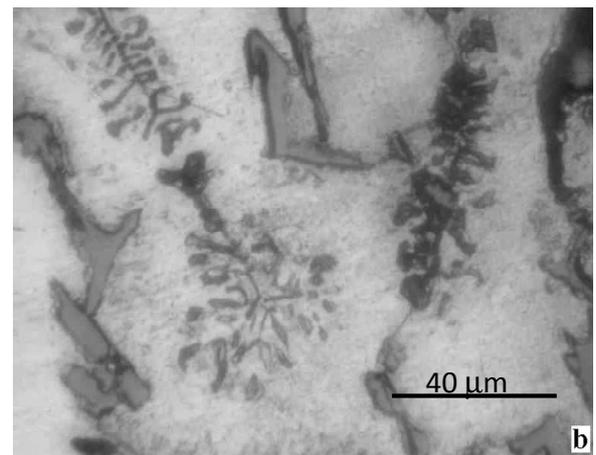
Fig. 5. The microphotos of matrix allows: a- allow ENACAlSi5Cu3; b- allow ENACAlSi7Cu2Mg
