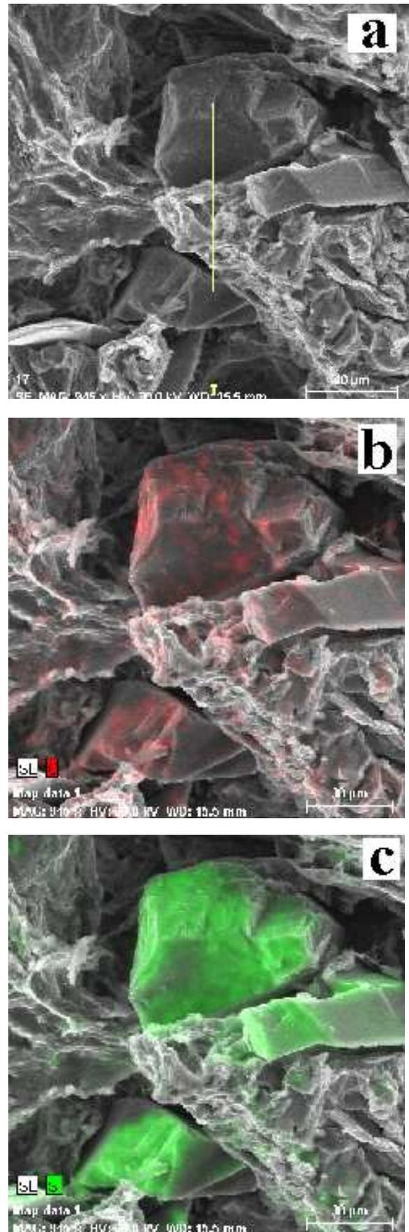
Fig. 7. The break imagines surface for ENACAlSi7Cu2Mg /particlae SiC (40  $\mu\text{m}$ ) surface:
