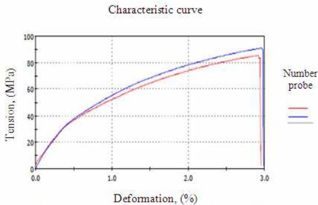
Fig. 3. Characteristic curve for the base alloy
