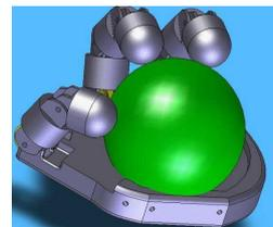
Fig. 9. The virtual model of the hand in solidWorks
