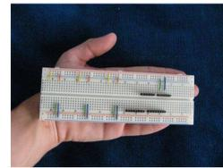
Fig. 12. The breadboard
