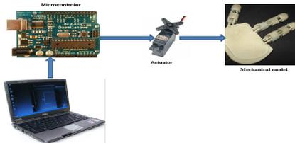
Fig. 10. The components of the control system
