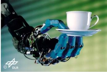
Fig.4.The DLR II robotic hand [1]
