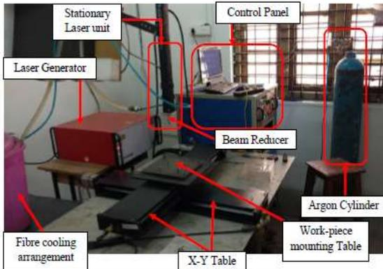
Fig. 2. Fiber laser system (SPI 400 CW, Laser Science Pvt. Ltd. Mumbai)
