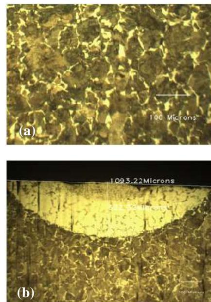
Fig. 4. Microstructure of (a) base metal and (b) laser treated samples at laser power of 260W, laser scan speed of 10 mm/s and stand-off distance of 270mm
