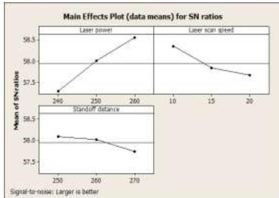
Fig. 3. Main effects of plot for S/N ratios
