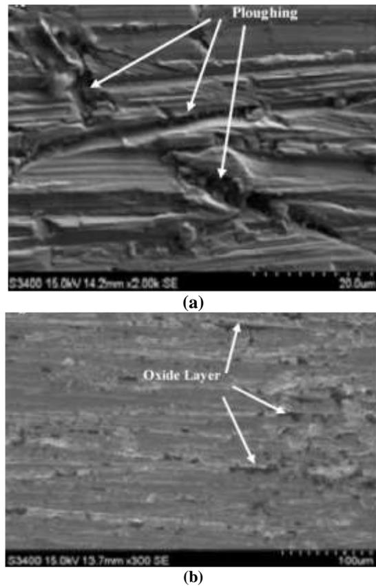
Fig 7. SEM images of wear scars of Ck45 steel samples at constant applied load of 30NW:- a) Base metal, b) laser treated sample at P = 260W, s = 10mm/s and f = 270mm
