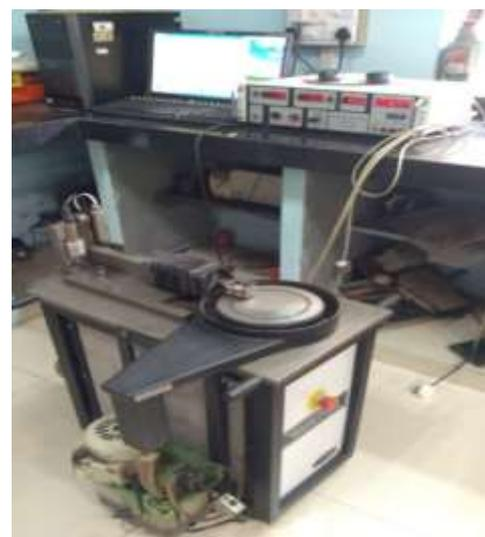
Fig. 5. Experimental set up of pin on disc for wear testing
