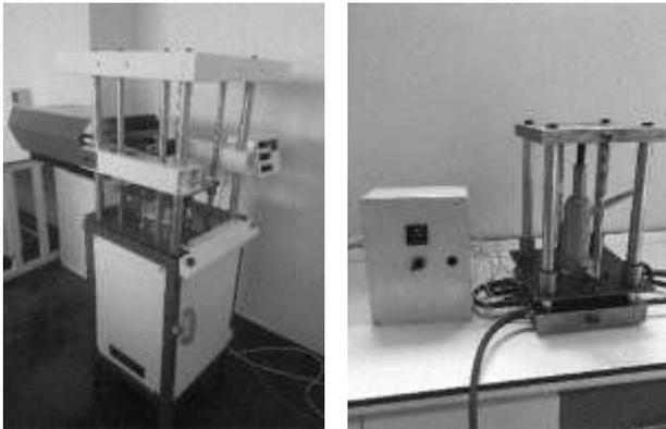
Fig.1. Lab-scale thermoforming machine and sample preparation mould respectively
