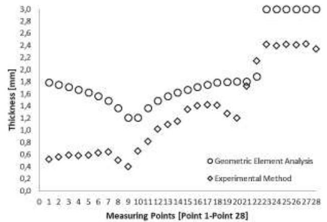
Fig. 5. Comparative thickness variation in conical thermoformed sample
