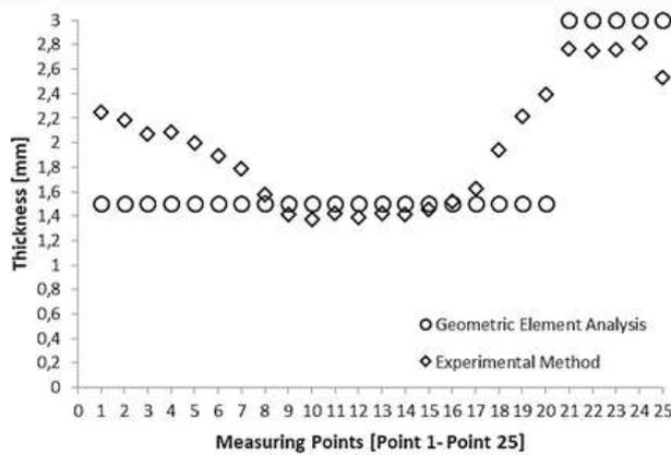
Fig. 4. Comparative thickness variation in spherical thermoformed sample
