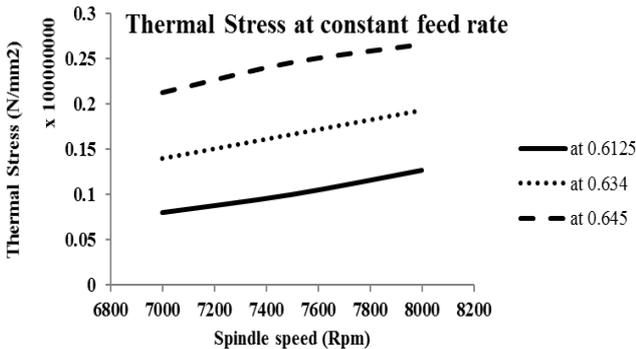
Fig. 6. Graph between thermal stress and spindle speed at constant feed per tooth
