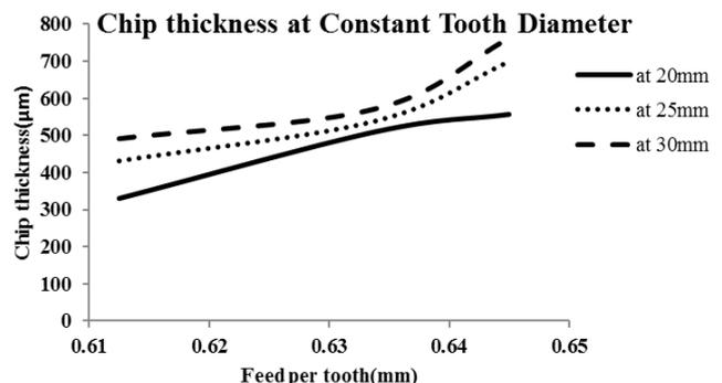
Fig. 10. Graph between chip thickness and feed per tooth at constant tooth diameter
