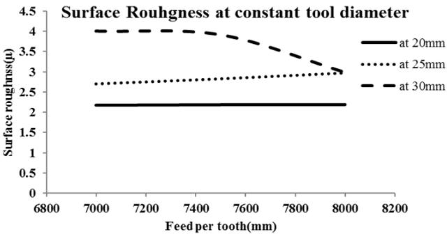
Fig.19. Graph between surface roughness and feed per tooth at constant depth of cut
