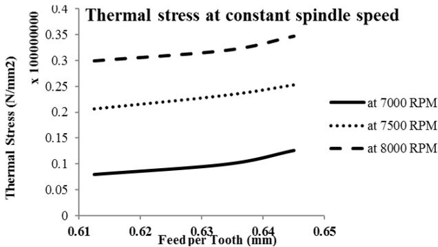
Fig. 5. Graph between thermal stress and feed per tooth at constant spindle speed
