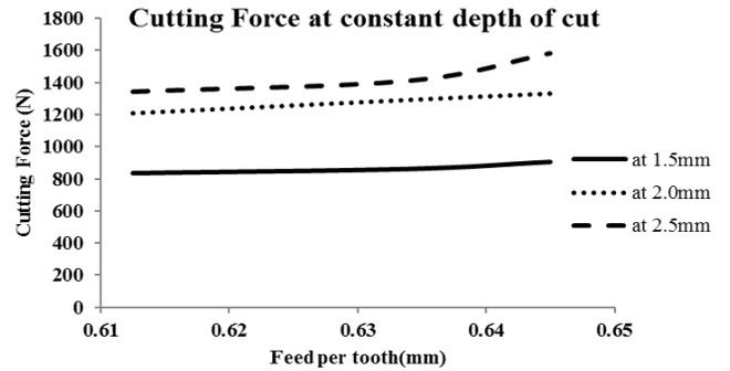
Fig. 15. Graph between cutting force and feed per tooth at constant depth of cut
