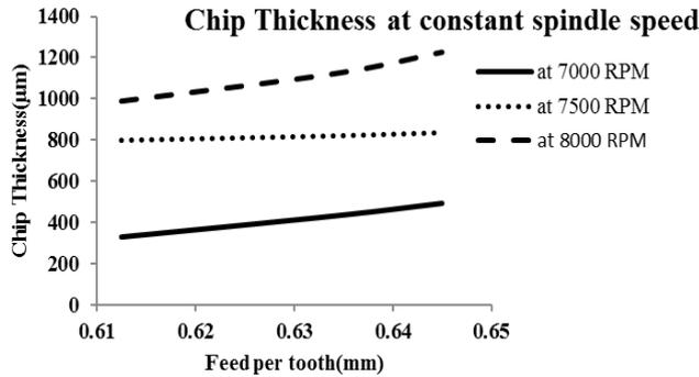
Fig. 12. Graph between chip thickness and feed per tooth at constant spindle speed
