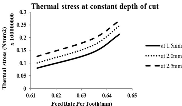
Fig. 8. Graph between thermal stress and feed per tooth at constant depth of cut
