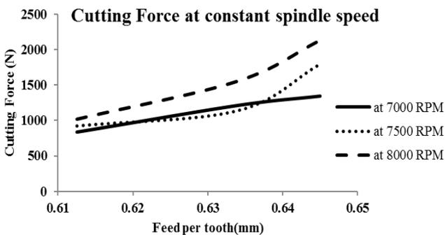
Fig. 13. Graph between cutting force and feed per tooth at constant spindle speed
