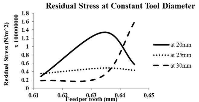
Fig. 3. Graph between residual stress and feed per tooth at constant tool diameter
