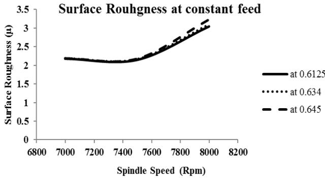
Fig.18. Graph between surface roughness feed and spindle speed at constant feed per tooth
