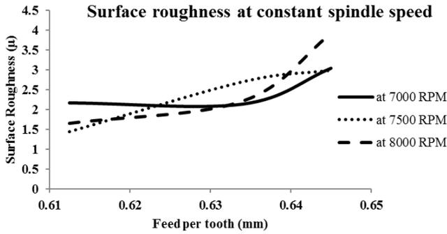
Fig. 17. Graph between surface roughness and per tooth at constant spindle speed
