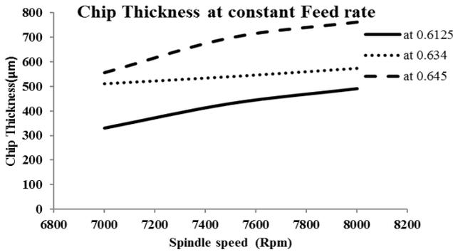
Fig. 11. Graph between chip thickness and spindle speed at constant feed per tooth
