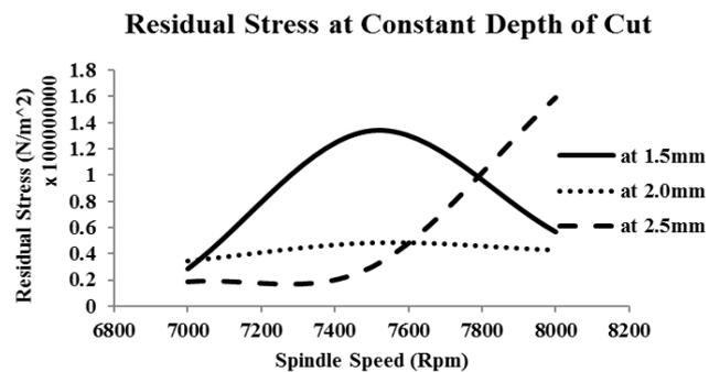
Fig. 4. Graph between residual stress and spindle speed at constant depth of cut
