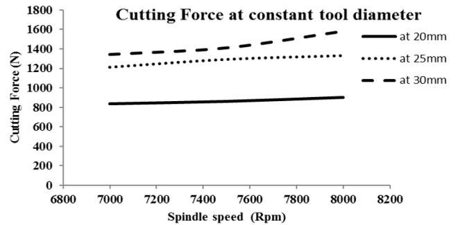
Fig. 16. Graph between cutting force and spindle speed at constant tool diameter
