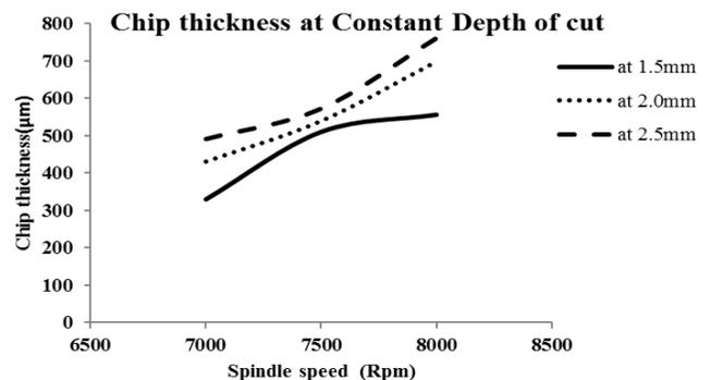
Fig. 9. Graph between chip thickness and spindle speed at constant depth of cut
