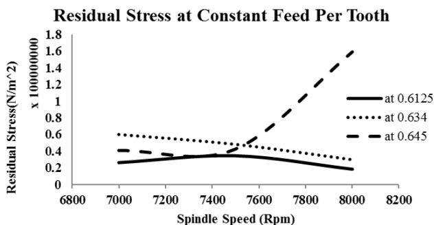
Fig. 1. Graph between residual stress and spindle speed at constant feed per tooth
