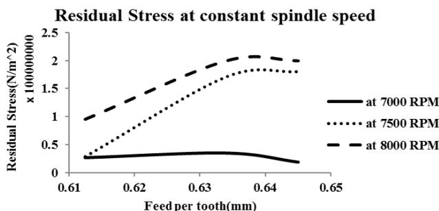
Fig. 2. Graph between residual stress and feed per tooth at constant spindle speed
