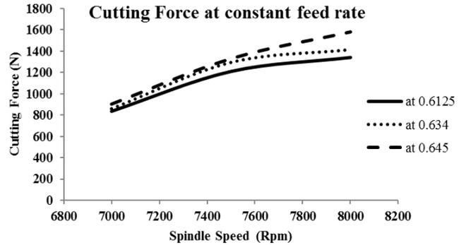
Fig. 14. Graph between cutting force and spindle speed at constant feed per tooth
