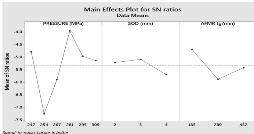
Fig. 5. Optimization plot for S/N ratios
