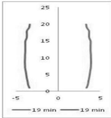
Fig. 12. Optimum deep hole profile
