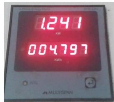
Fig. 6. Power measurement
