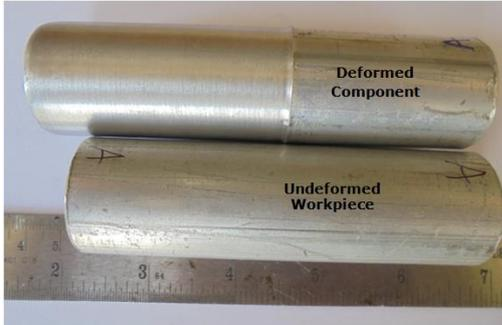
Fig. 8. Deformed samples
